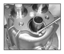
12. If the crankcase oil seals (15) are to be replaced, they can be removed by prying loose with a screwdriver. Take care not to make contact with the plunger (8) and pry out the oil seals from their housing. Seals should not be reinstalled until after step #16.
